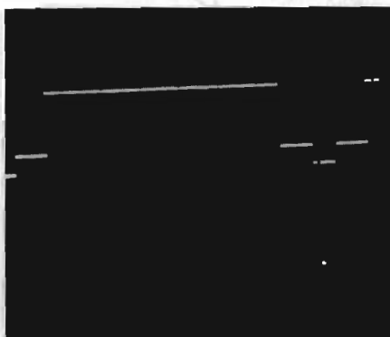
Photo 4: Oscilloscope trace of the output video showing one video frame.
