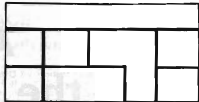
Figure 2: Full-size layout of the amplifier board. Make the board by etching the lines shown to divide the board into eight segments as shown.
